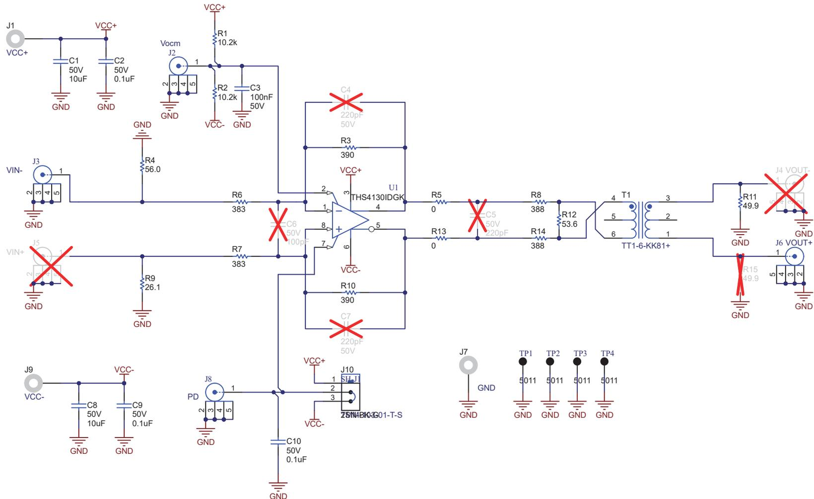
Figure 3-1. Schematic with Example Configuration Using the THS4130
