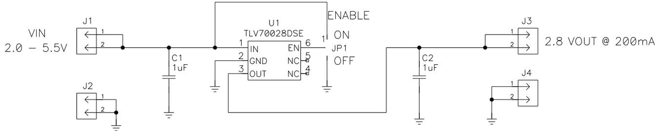
Figure 4. TLV700xxEVM-463 Schematic
