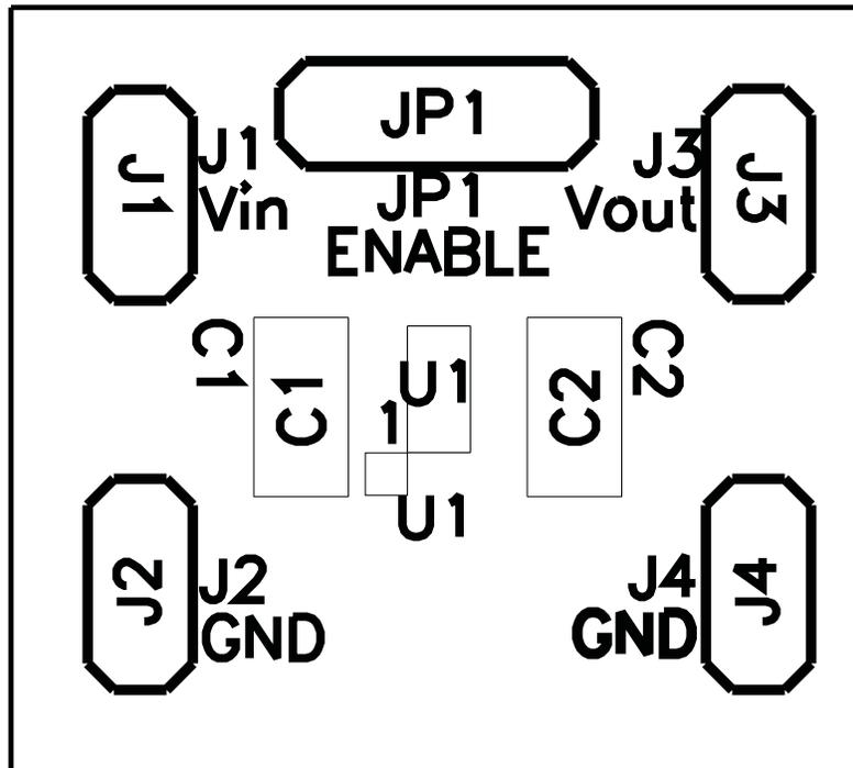
Figure 1. Assembly Layer
