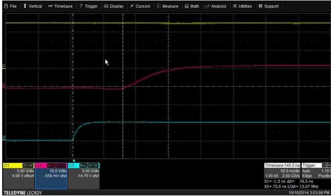
Figure 20. LI, LO Turn-On Propagation Delay
