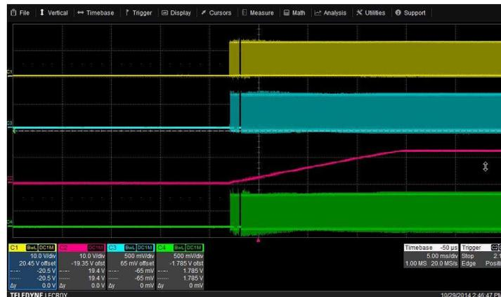
Figure 28. UCC28950 Burst-Mode Function During Soft Start
