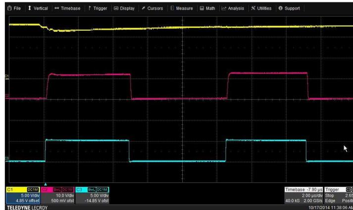
Figure 22. VDD Drop On First Bootstrap Capacitor Charging
