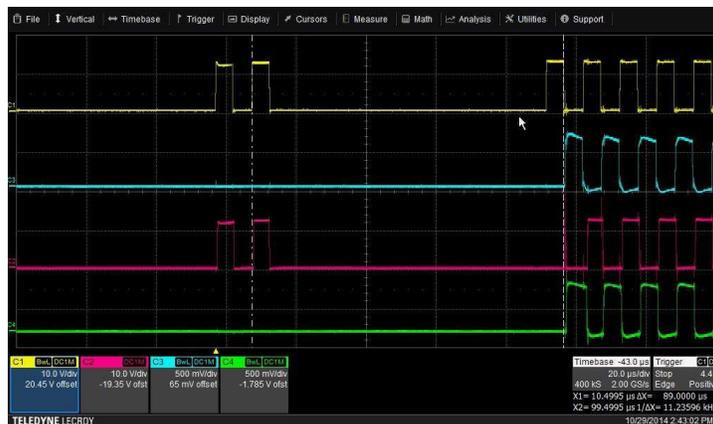
Figure 26. Q<sub>g</sub> Measurement During Startup
