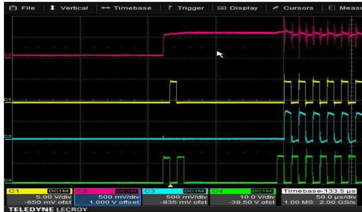
Figure 25. HB and HO Measurement During Start Up
