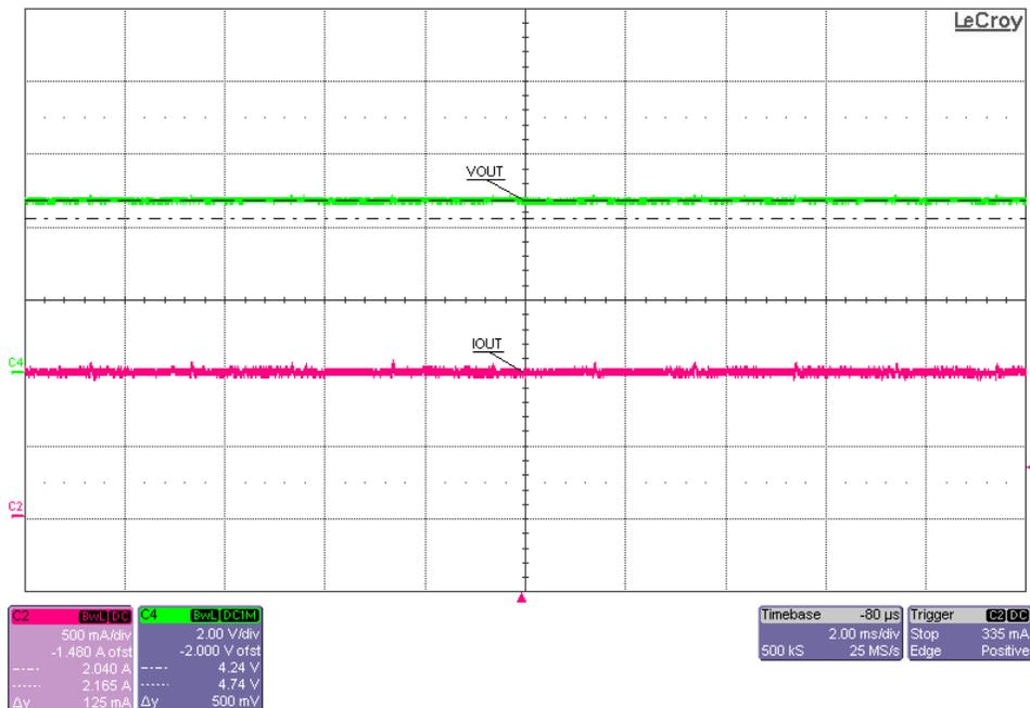
Figure 2. bq51020 in Steady State Operation with bq24250
