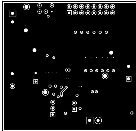
Figure 20. TPS53317AEVM-726 Layer 2 (Top View)
