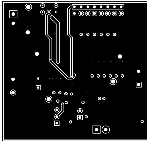
Figure 21. TPS53317AEVM-726 Layer 3 (Top View)
