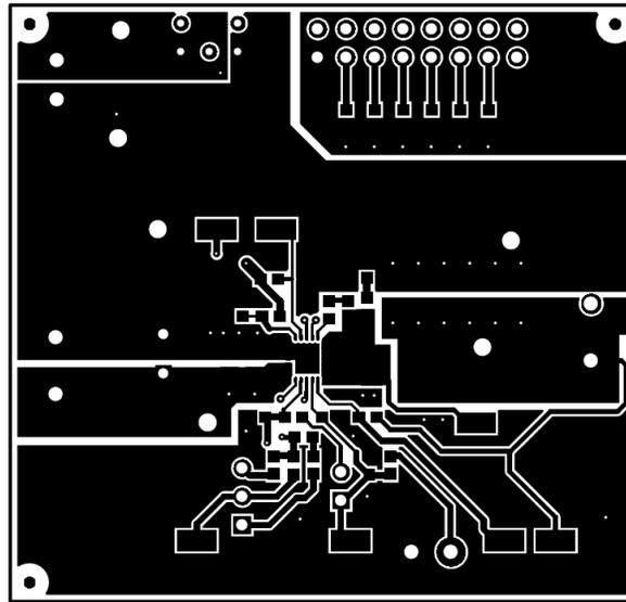
Figure 19. TPS53317AEVM-726 Top Copper (Top View)
