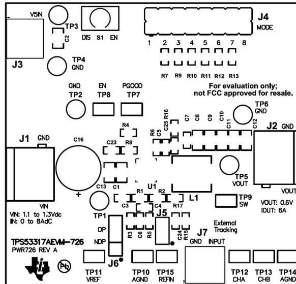
Figure 17. TPS53317AEVM-726 Top Layer Assembly Drawing (Top View)
