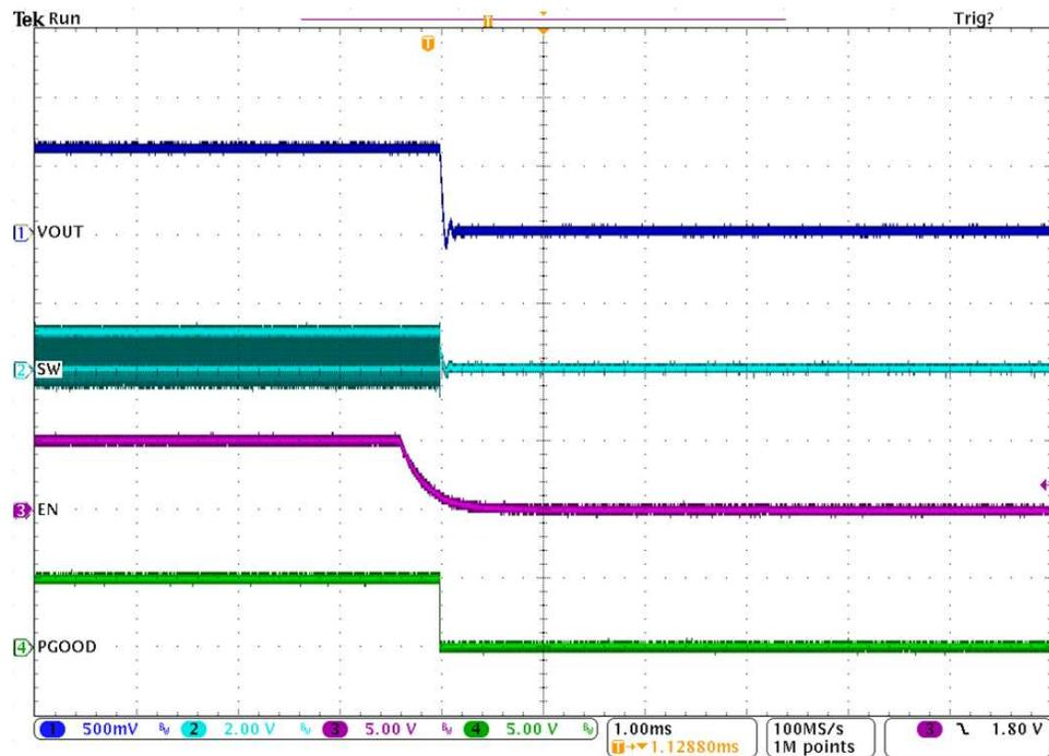
Figure 13. Turn-Off Waveform
