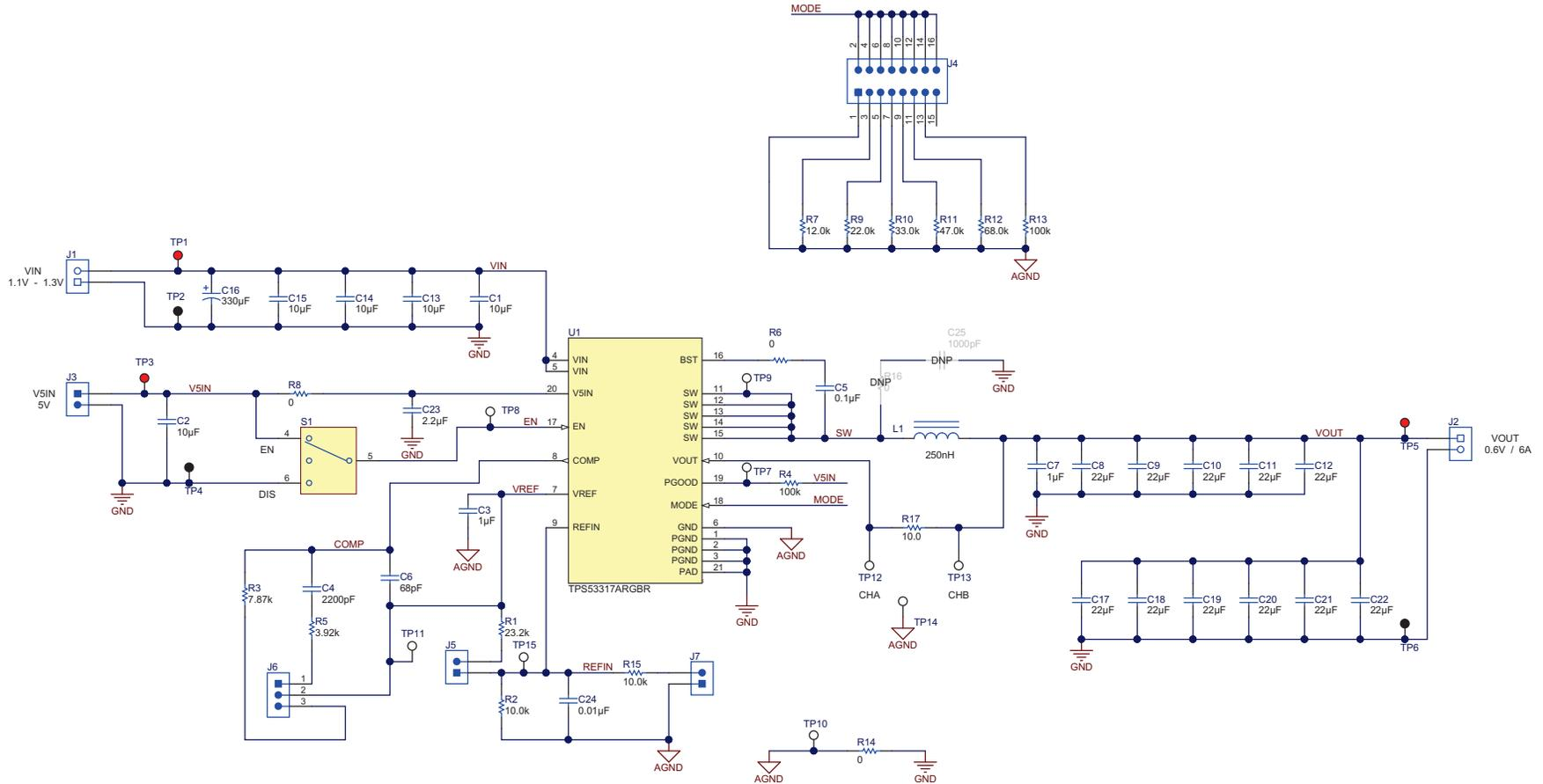
Figure 1. TPS53317AEVM-726 Schematic
