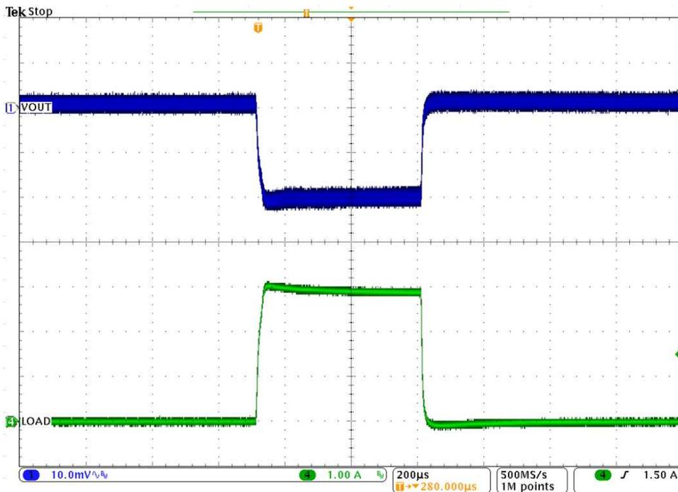
Figure 7. Output Load 0-A to 3-A Transient with Droop
