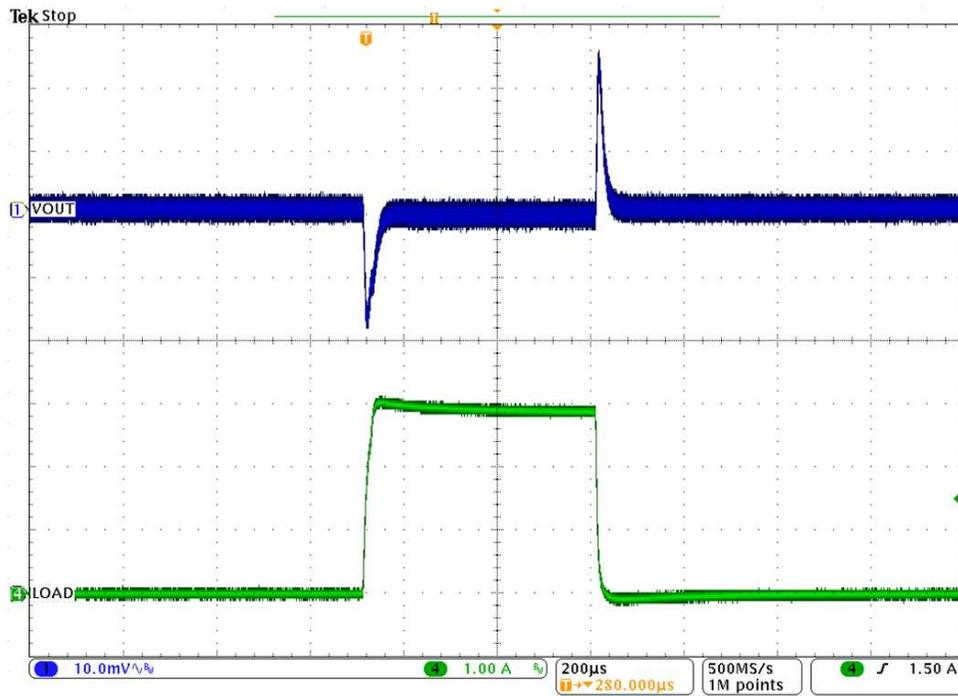
Figure 6. Output Load 0-A to 3-A Transient
