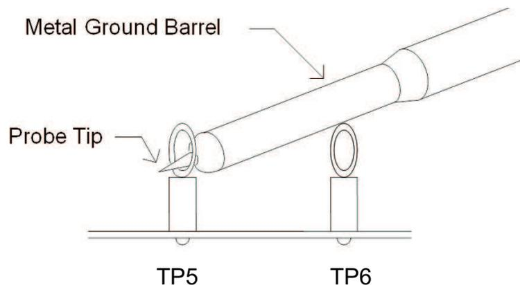
**Figure 2. Tip and Barrel Measurement for VOUT Ripple**
