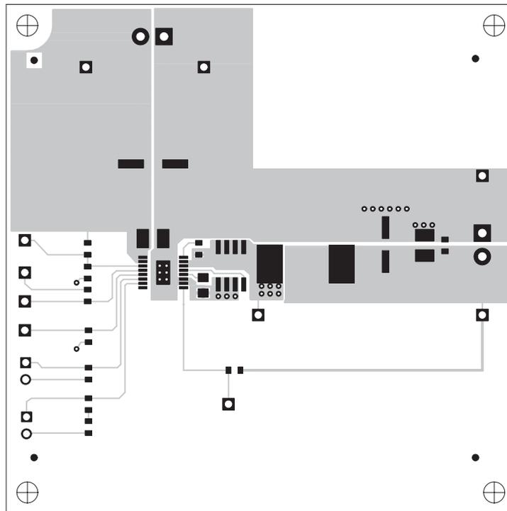
Figure 3–2. Bottom Side Layout (looking from top side)
