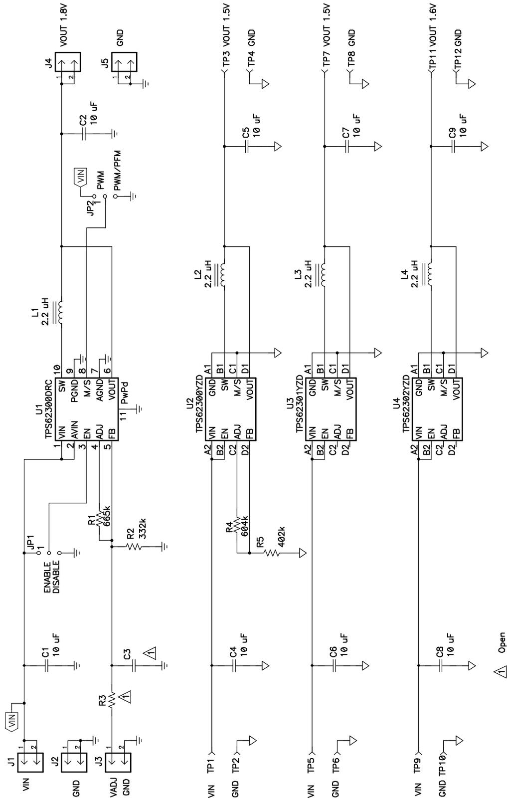
Figure 4. TPS6230xEVM-085 Schematic
