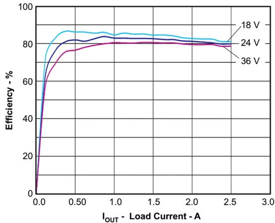
NOTE:  $V_{IN} = 18\text{ V}, 24\text{ V}, \text{ and } 36\text{ V}$ ,  $V_{OUT} = 3.3\text{ V}$ ,  $I_{OUT} = 0.125\text{ A to } 2.5\text{ A}$
