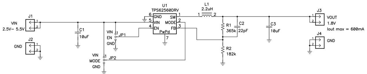
**Figure 8. TPS62560EVM-330 Schematic**
