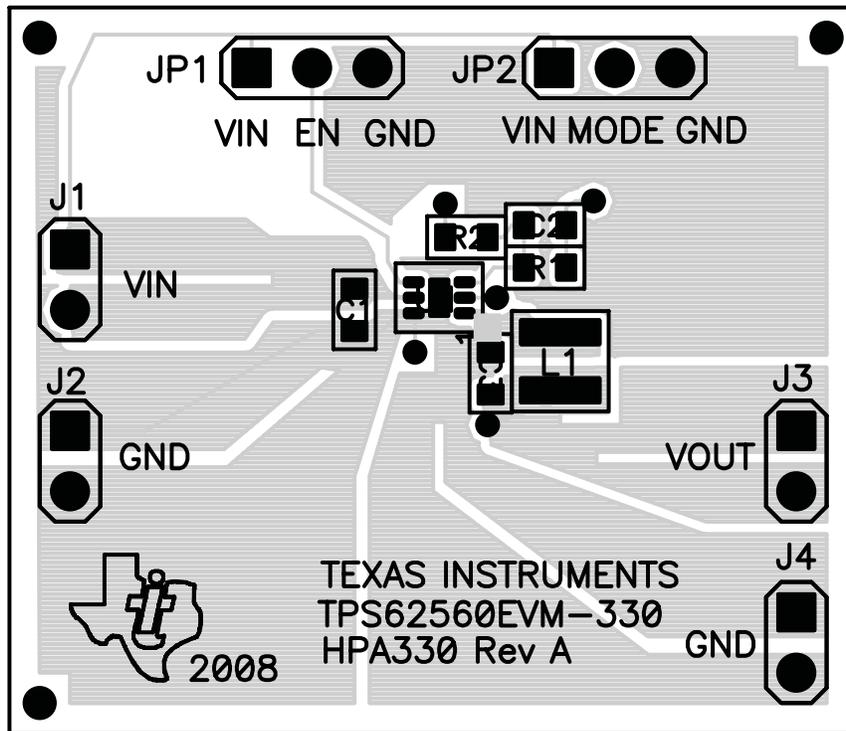
Figure 5. Assembly Layer
