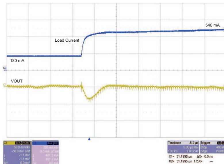
**Figure 4. Load Transient, 180-mA to 540-mA Step**
