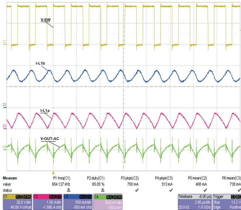
Figure 5. PWM Operation at 750 mA with  $V_{IN} = 24V$
