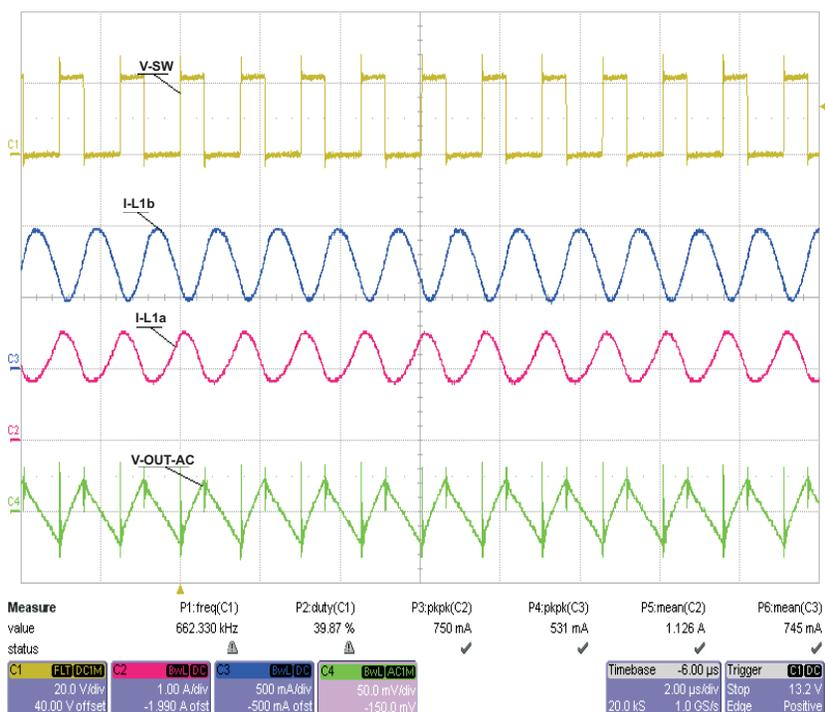
Figure 4. PWM Operation at 750 mA with  $V_{IN} = 9V$
