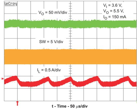
Figure 10. TPS61251 EVM Output Voltage Ripple at 150mA
