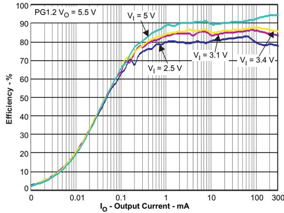
Figure 2. TPS61251 EVM Efficiency vs Load Current
