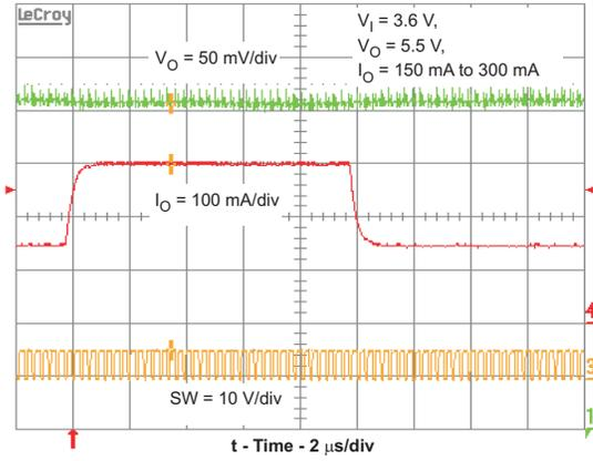
Figure 6. TPS61251 EVM Load Transient Response, CCM Mode
