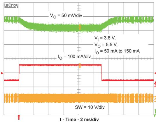
Figure 4. TPS61251 EVM Load Transient Response, PFM Mode
