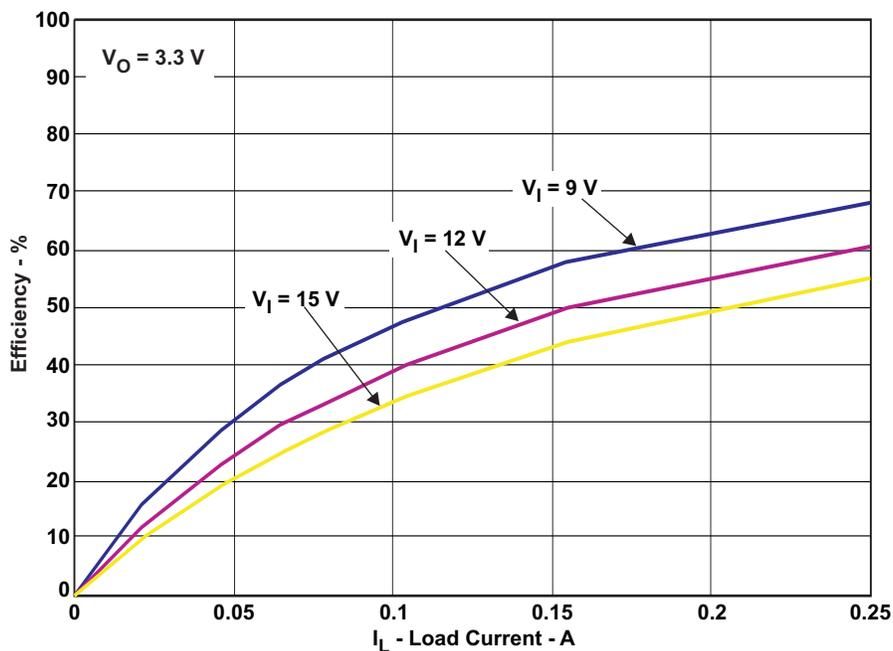
Figure 3. Light-Load Efficiency vs Input Voltage at 25°C
