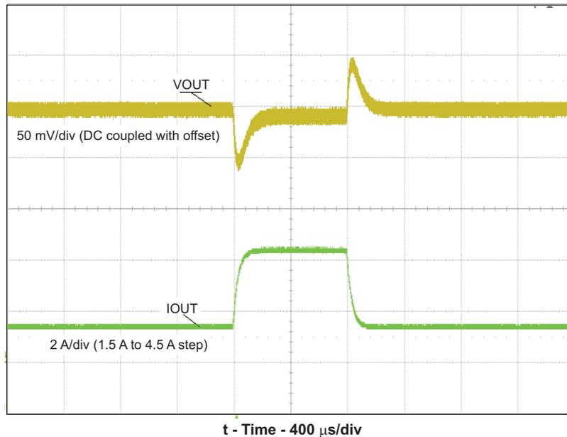
Figure 8. 3.3-V TPS84620EVM-692 Transient Response at 25°C
