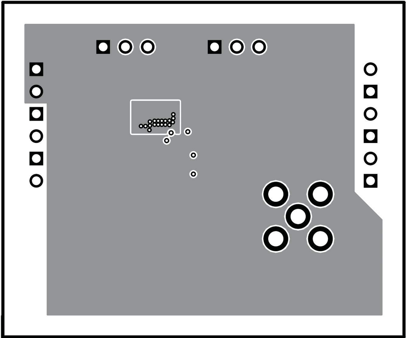
Figure 19. TLV62065EVM Internal Layer 2, X-Ray View From Top
