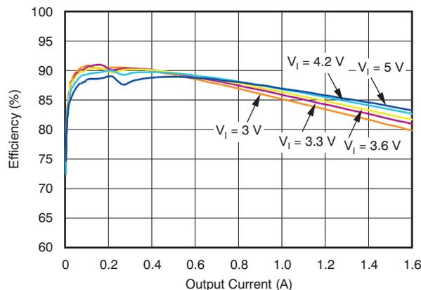
Figure 3. TLV62065 Efficiency vs Load Current, PFM Mode
