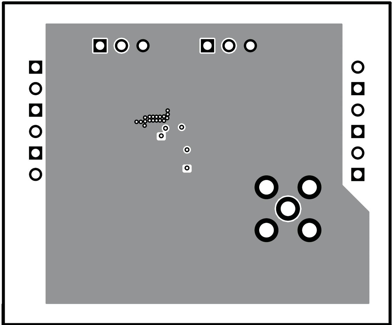
Figure 18. TLV62065EVM Internal Layer 1, X-Ray View From Top
