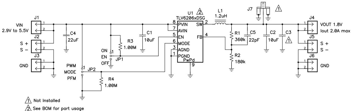
Figure 1. TLV62065EVM Schematic
