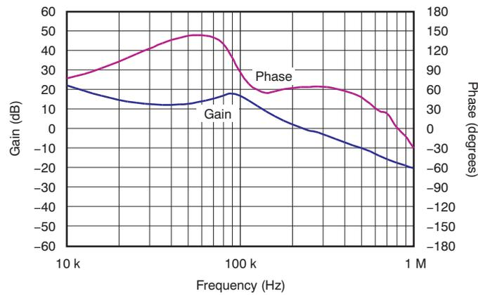
Conditions:  $V_{IN} = 5\text{ V}$ ,  $V_{OUT} = 1.8\text{ V}$ ,  $I_{OUT} = 1.6\text{ A}$ ; bandwidth: 241 kHz, phase margin:  $66^\circ$
