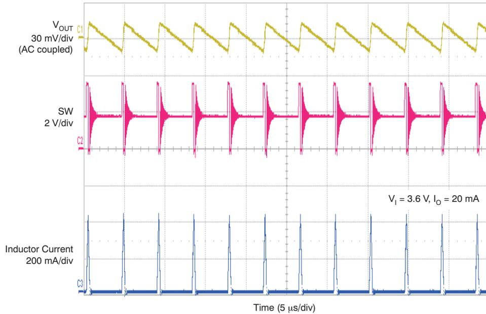
**Figure 9. TLV62065 Output Voltage Ripple, PFM Mode**
