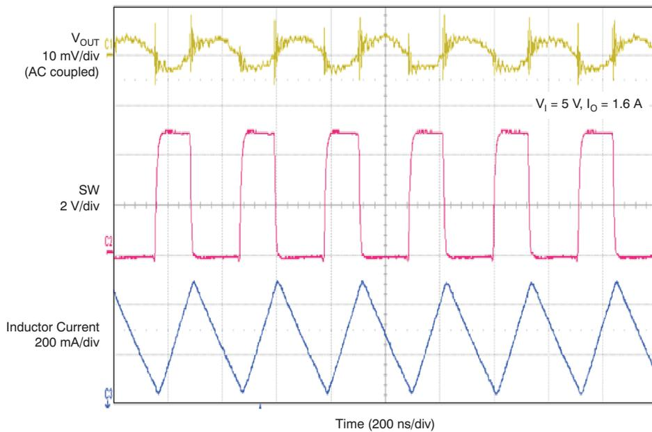
**Figure 10. TLV62065 Output Voltage Ripple, PWM Mode**
