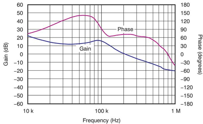
Conditions:  $V_{IN} = 3.6$  V,  $V_{OUT} = 1.8$  V,  $I_{OUT} = 1.6$  A; bandwidth: 213 kHz, phase margin: 73°
