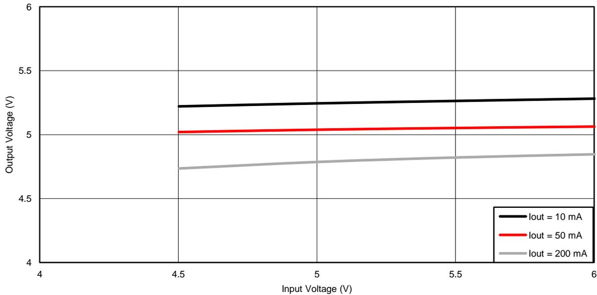
Figure 3. TPS55010EVM-009 Line Regulation,  $V_{IN} = 5\text{ V}$
