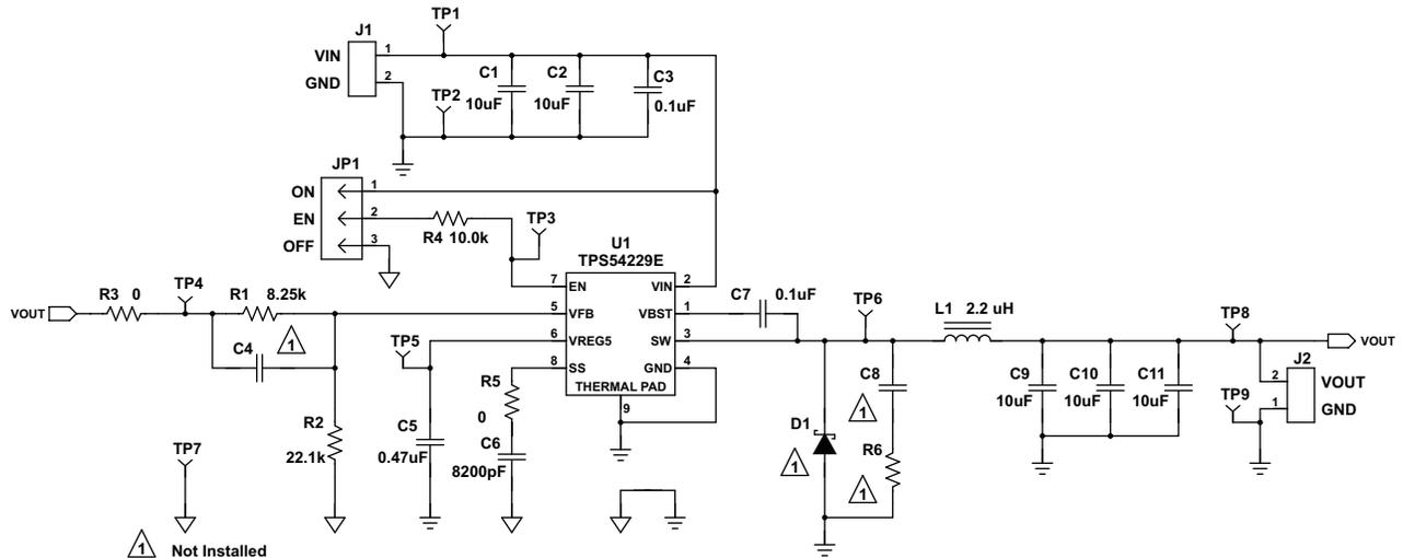
Figure 20. TPS54229EEVM-056 Schematic Diagram
