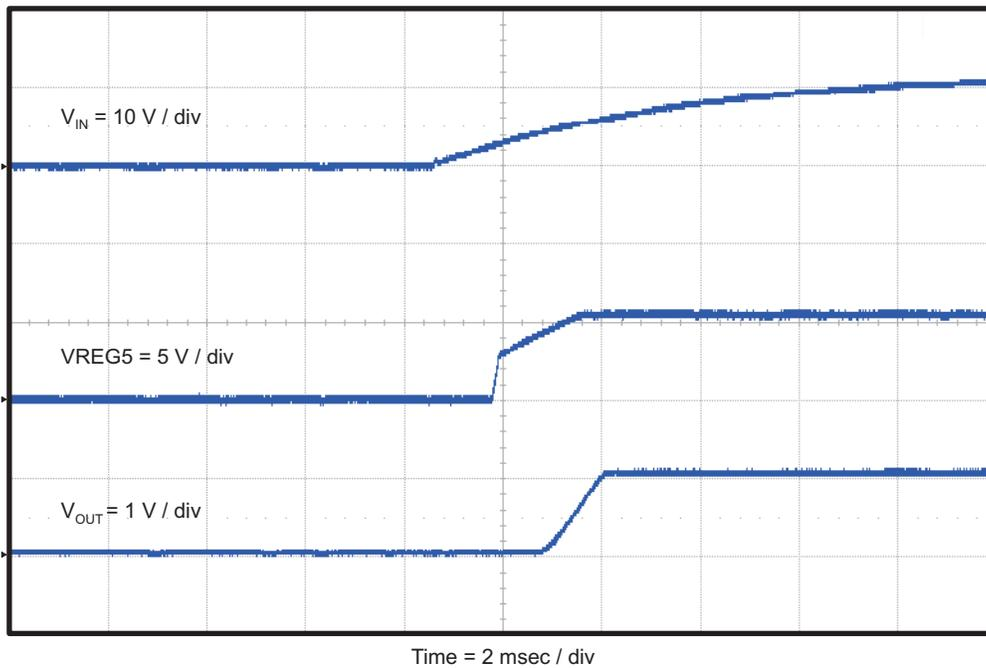
**Figure 12. TPS54229EEVM-056 Start-Up Relative to  $V_{IN}$  With VREG5**
