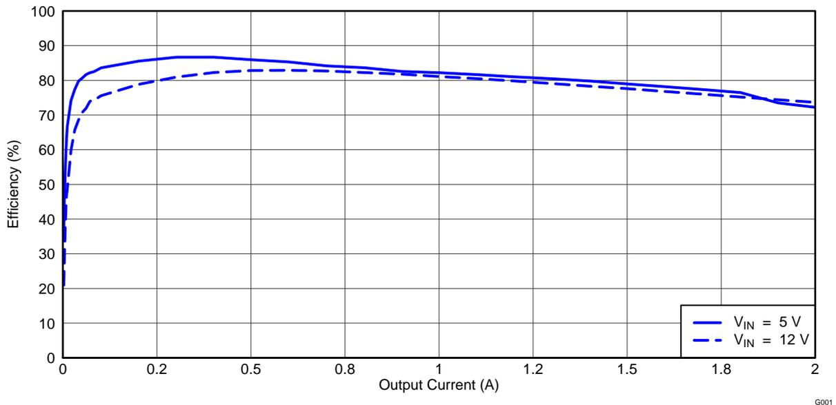
**Figure 1. TPS54229EEVM-056 Efficiency**
