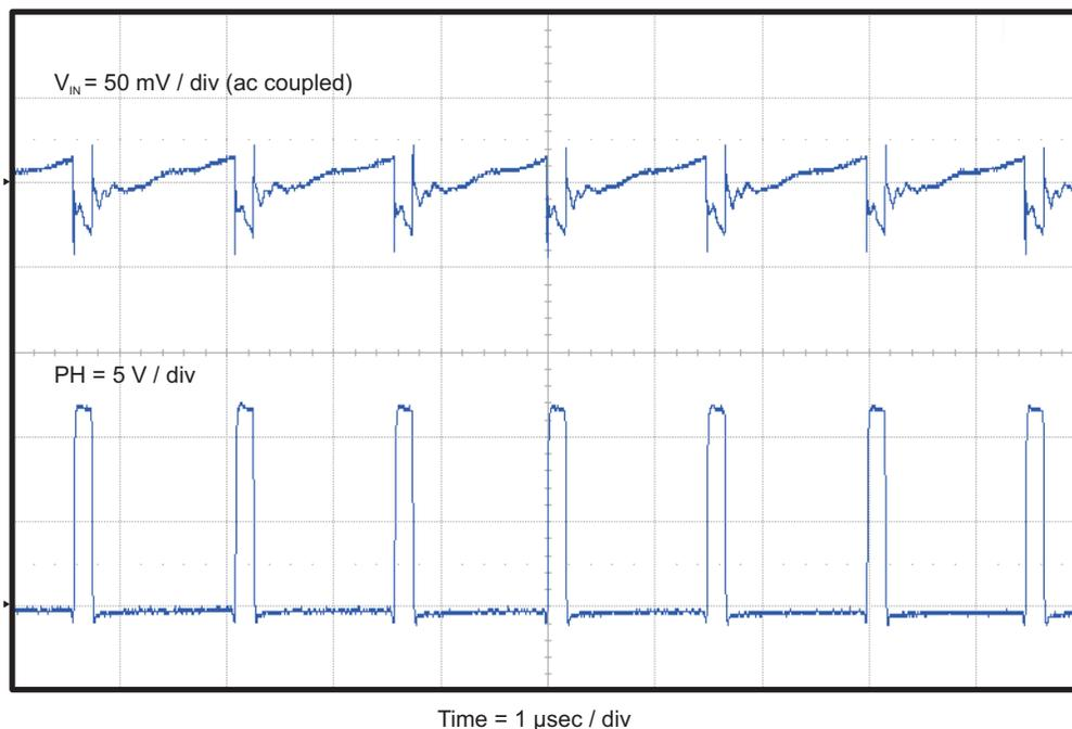
Figure 10. TPS54229EEVM-056 Input Voltage Ripple
