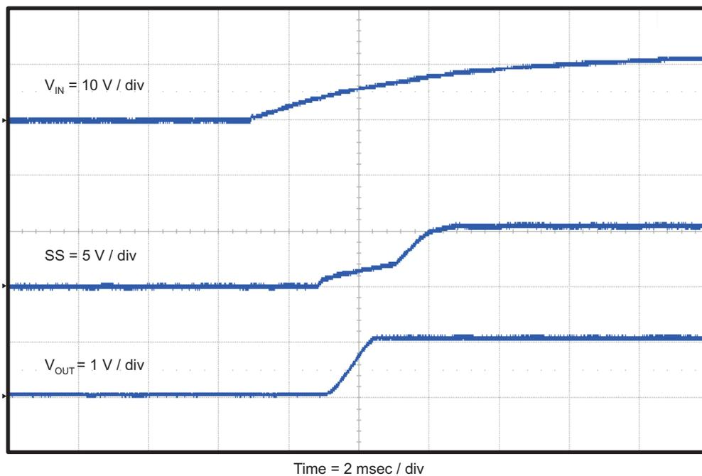
Figure 11. TPS54229EEVM-056 Start-Up Relative to  $V_{IN}$  With SS
