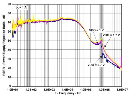
Figure 2. TPS7A8101 PSRR for Variable Dropout Voltage, lout=1 A
