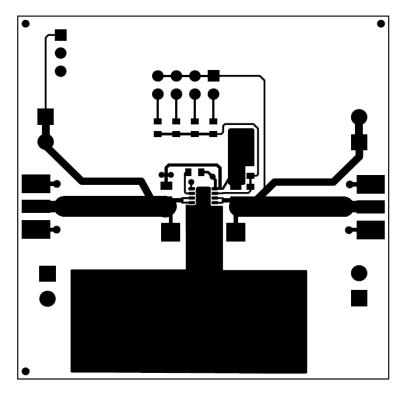
Figure 7. Top Layer Routing
