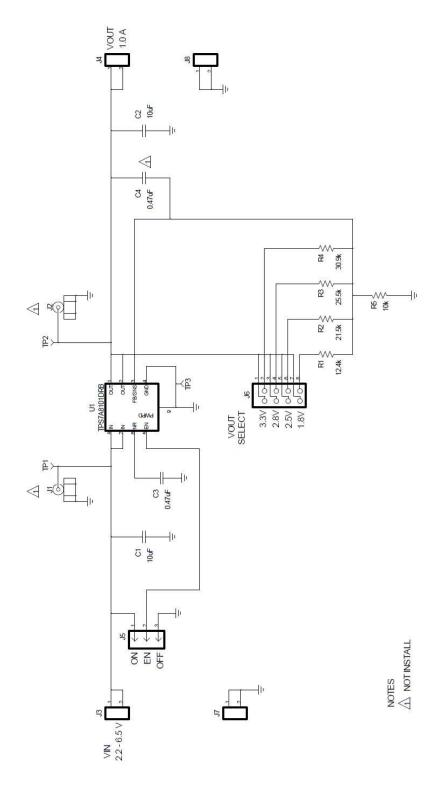
Figure 9. TPS7A8101EVM Schematic
