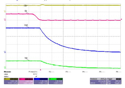
Figure 4. TPS7A8101 Shutdown with 3.3- $\Omega$  Load
