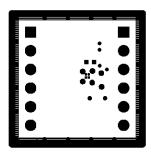
Figure 9. SMP-TPS7A3001-MVK Board Solder Mask – Bottom Side
