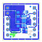
Figure 12. SMP-TPS7A3001-MVK Board Layer 1 - Top Side
