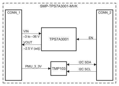
Figure 2. SMP-TPS7A3001-MVK Block Diagram
