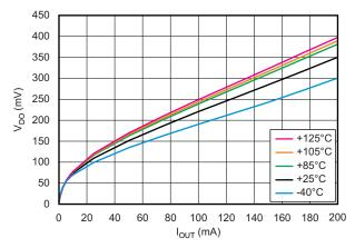
Figure 3. TPS7A3001 Dropout Voltage Versus Output Current
