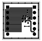
Figure 7. SMP-TPS7A3001-MVK Board Layer 4 – Bottom Side
