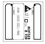
Figure 11. SMP-TPS7A3001-MVK Board Silkscreen – Bottom Side
