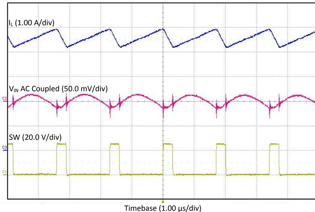
Figure 11. TPS55340EVM-017  $V_{IN} = 5\text{-V}$  Input Voltage Ripple
