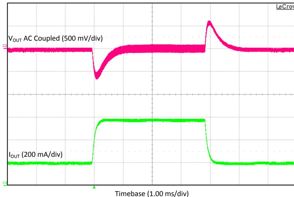
Figure 5. TPS55340EVM-017 V<sub>IN</sub> = 12-V Transient Response
