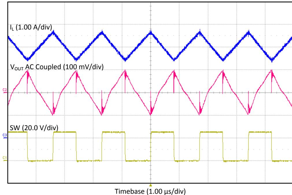
**Figure 8. TPS55340EVM-017  $V_{IN} = 12$ -V Output Ripple**
