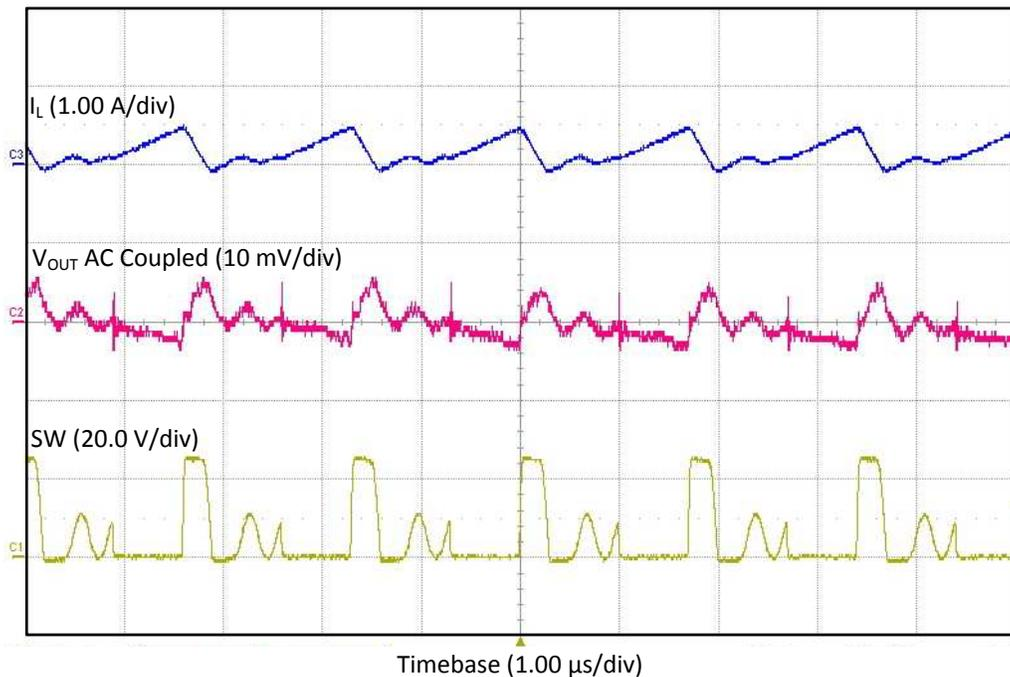
**Figure 9. TPS55340EVM-017 DCM Output Ripple**
