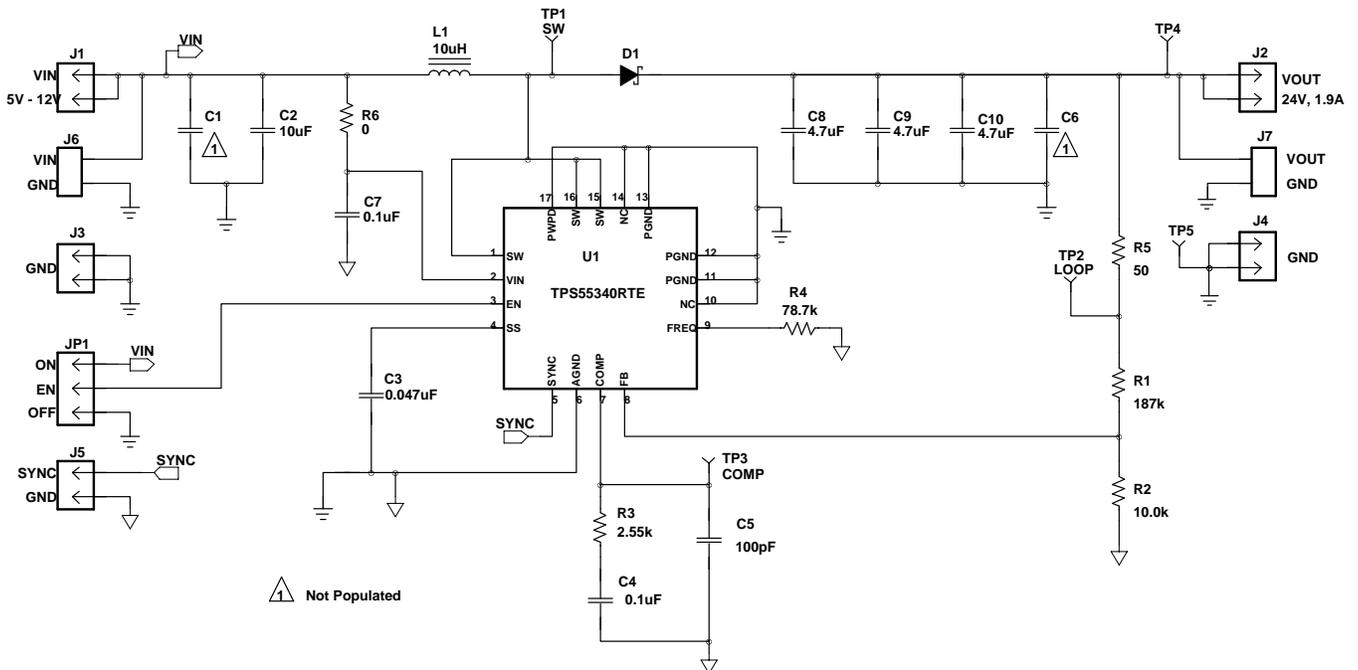
Figure 22. TPS55340EVM-017 Schematic
