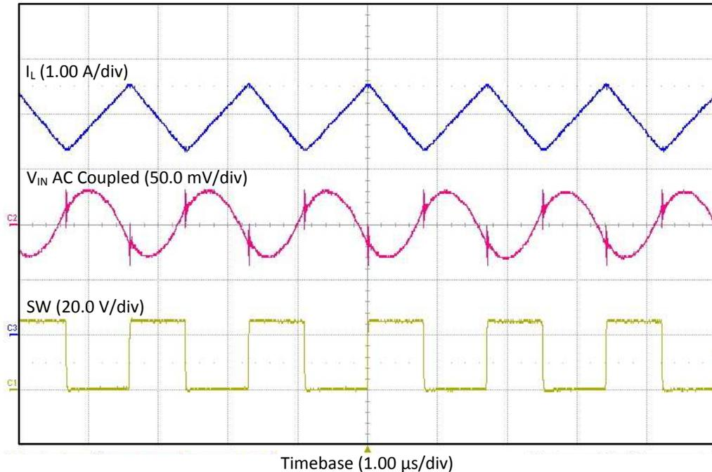
Figure 12. TPS55340EVM-017  $V_{IN} = 12$ -V Input Voltage Ripple
