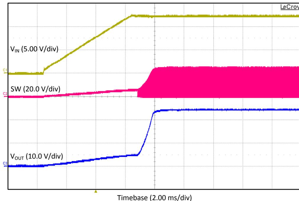
Figure 15. TPS55340EVM-017 Power Up With  $V_{IN}$
