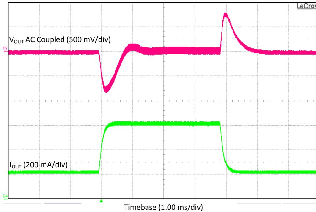
Figure 4. TPS55340EVM-017 V<sub>IN</sub> = 5-V Transient Response
