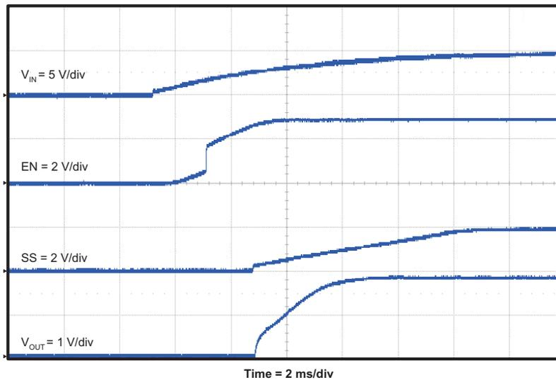
**Figure 9. TPS5432EVM-116 Start-Up Relative to  $V_{IN}$**
