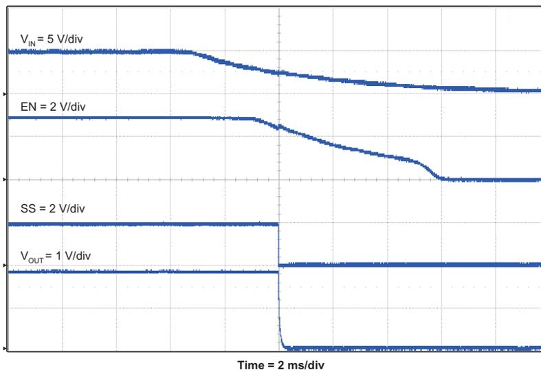
Figure 11. TPS5432EVM-116 Shut Down Relative to  $V_{IN}$
