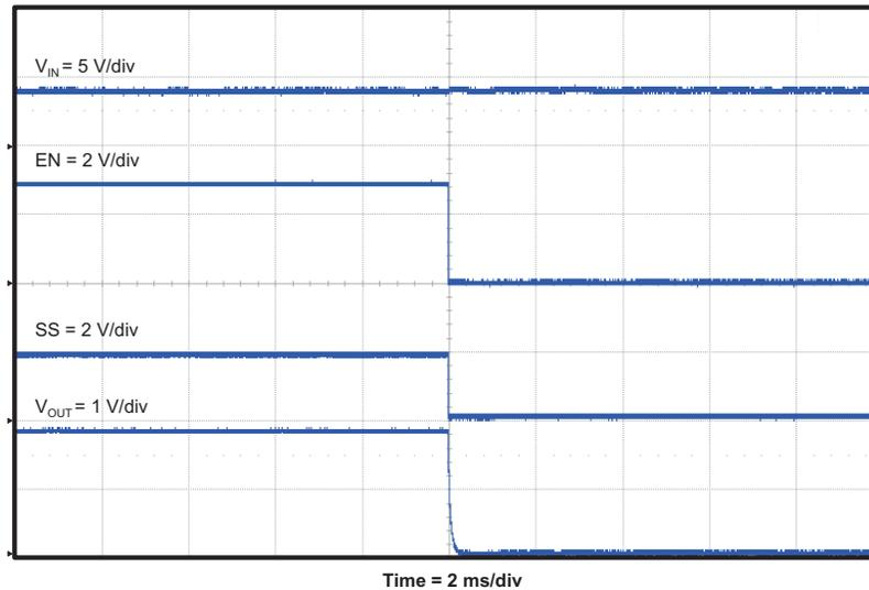
**Figure 12. TPS5432EVM-116 Shut Down Relative to EN**
