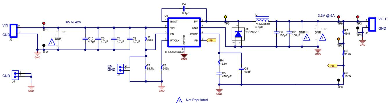
**Figure 2. TPS54540EVM-558 Schematic**
