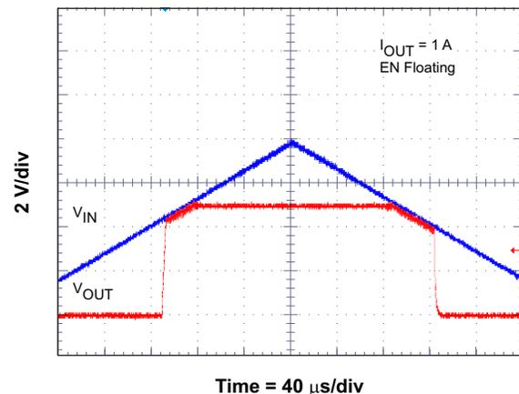
Figure 21. Low Dropout Start Up and Shutdown
