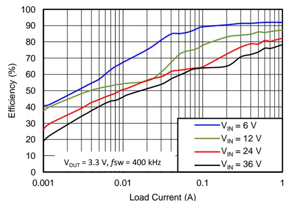
**Figure 4. Light-Load Efficiency**
