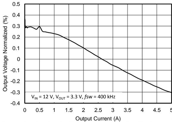
Figure 5. Regulation Versus Output Current
