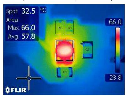
Figure 1. Thermal Performance ( $V_{IN} = 5 \text{ V}$ ,  $I_{OUT} = 3000 \text{ mA}$ )
