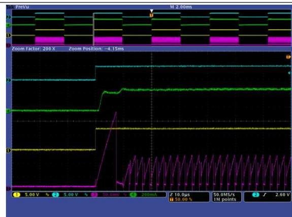
Ch1: DDRV voltage; Ch2: PWM input,
