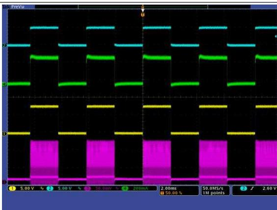
Ch1: DDRV voltage; Ch2: PWM input, TP3;
