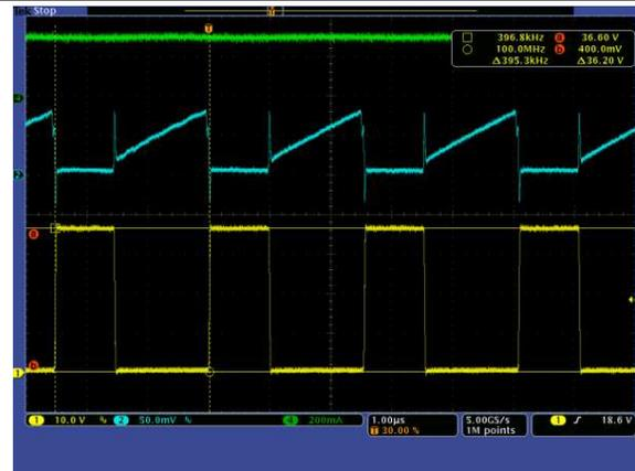
Ch1: Q2 Drain voltage;
