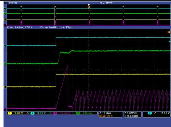
Ch1: DDRV voltage; Ch2: PWM input, TP3;
