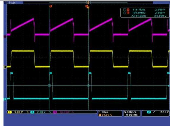
Ch1: GATE voltage; Ch2: SYNC input, TP2;
