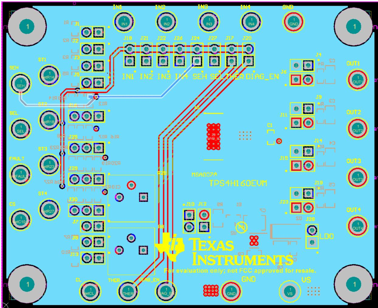
Figure 4. TPS4H160-Q1EVM Third Layer VCC (Top View)
