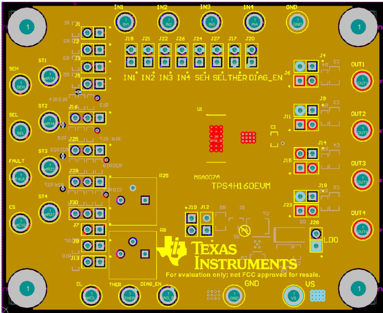
Figure 3. TPS4H160-Q1EVM Second Layer GND (Top View)
