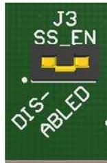
**Figure 19. Spread Spectrum Enable Jumper Configuration**
