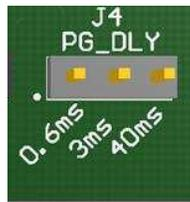
**Figure 20. Power-Good Delay Selection Jumper Configuration**
