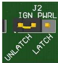
**Figure 18. Power-Latch Jumper Configuration**
