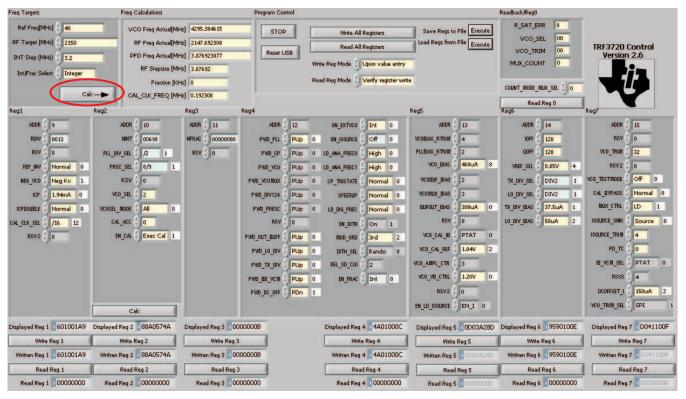
12. To change frequencies, enter the desired operating frequency in the RF Target (MHz) control. The GUI automatically calculates resulting frequencies to display in the Freq Calculations display. It also automatically calculates values for the necessary register settings and writes those values to the device. The calculated register entries are highlighted in blue.
