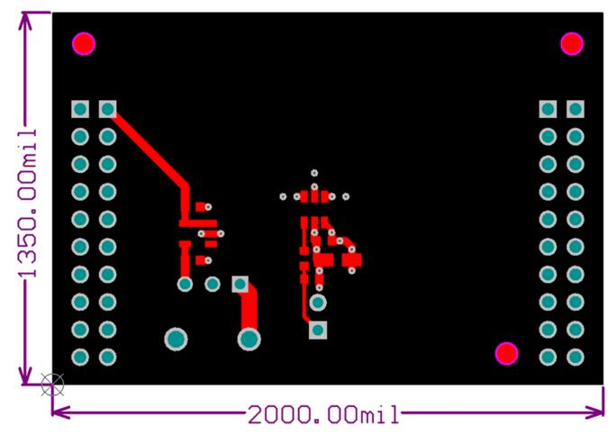
Figure 4-2. Top Layer Routing
