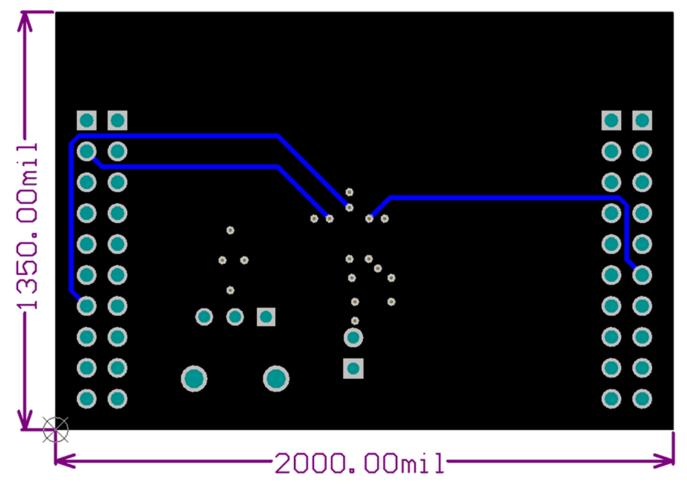
Figure 4-5. Bottom Layer Routing
