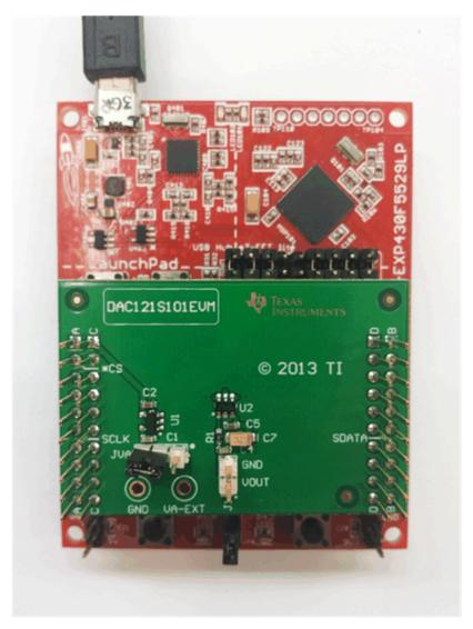
Figure 3-1. DAC121S101EVM Attached to MSP430
