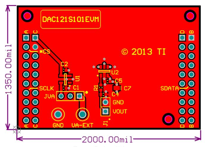
Figure 4-1. Top Assembly Layer
