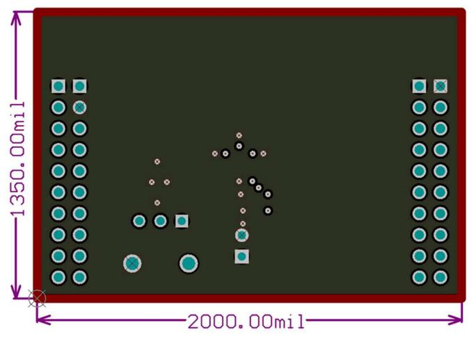
Figure 4-4. Ground Layer Routing
