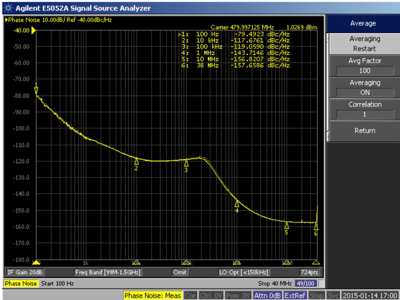
Figure 14. Default Mode vs. Fpd = 20 MHz and 4x Higher Charge Pump Gain
