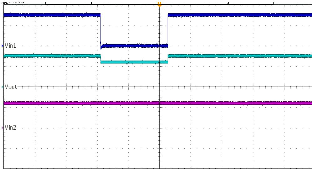
**Figure 6. ORing Application – Higher Supply Switchover**
