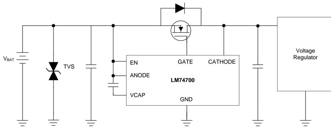
**Figure 1. LM74700EVM Typical Application Circuit**
