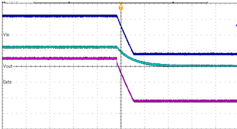
Figure 4. Reverse Polarity 12 V to -12 V
