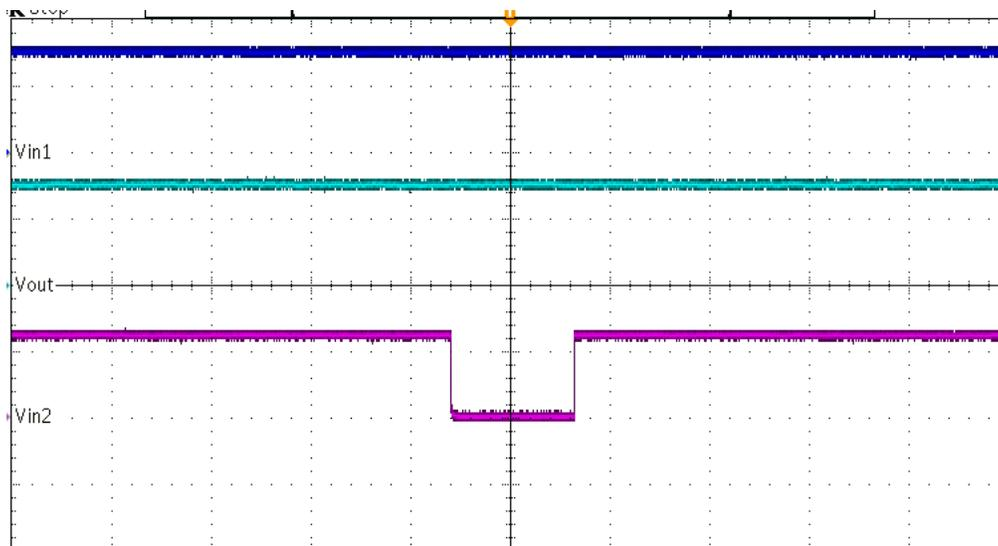
**Figure 7. ORing Application 12-V – Lower Supply Test**
