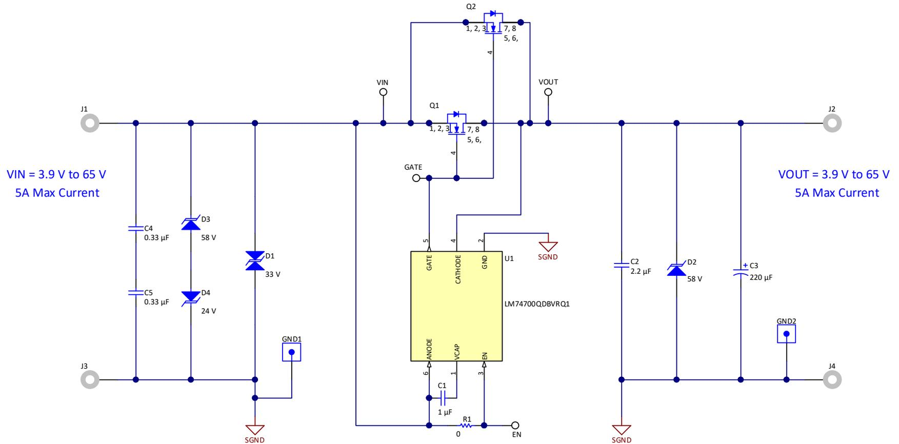
Figure 3. LM74700EVM Schematic
