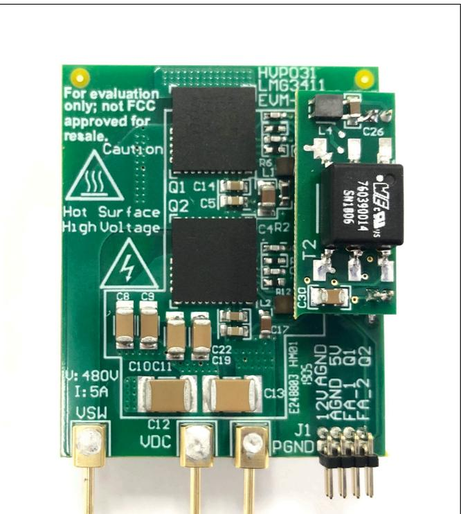
Figure 5. Back Side View of LMG3411EVM-031 in Isolated Power Supply Configuration
