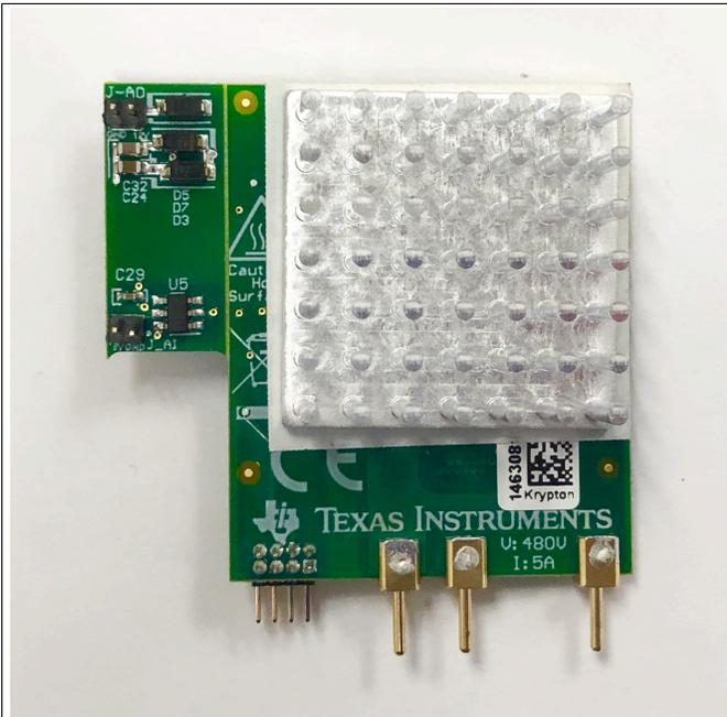
Figure 2. Top Side View of LMG3411EVM-031
