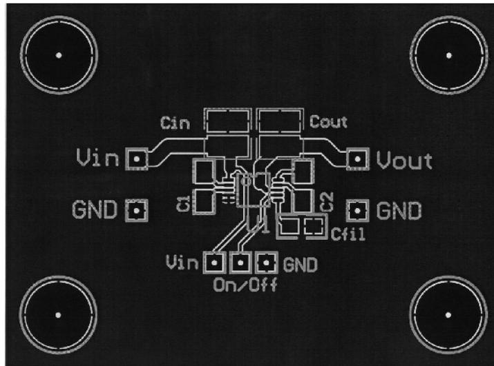
Figure 2. Typical Layout, Top View (magnification 1.5X)
