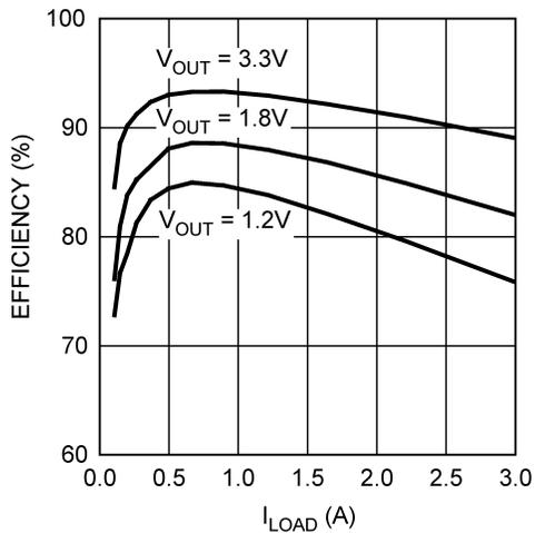
Figure 1. Efficiency vs.  $I_{LOAD}$  ( $V_{IN} = 5V$ )
