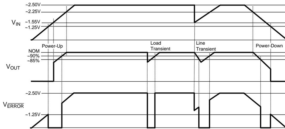
**Figure 5. ERROR Flag when Pull-Up is from V<sub>IN</sub>**
