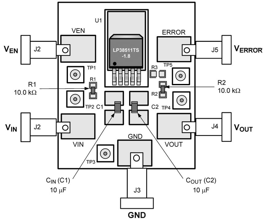
Figure 7. Evaluation Board Component and Pin Layout
