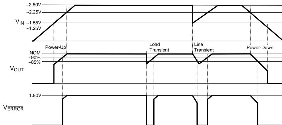
**Figure 4.  $\overline{ERROR}$  Flag when Pull-Up is from  $V_{OUT}$**
