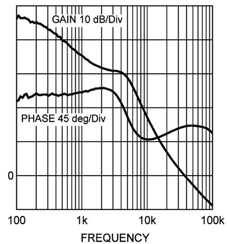
Figure 5. Overall Loop Gain and Phase ( $I_{OUT} = 3A$ )
