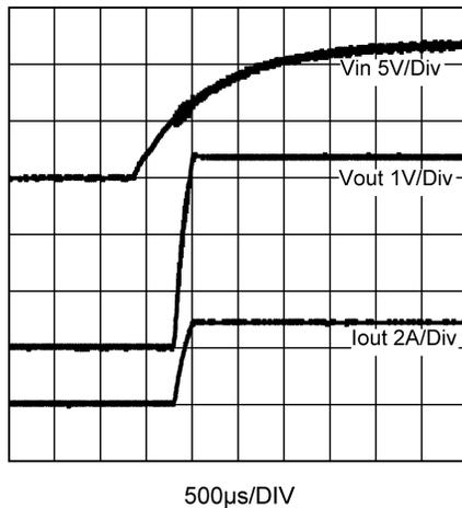
Figure 2. Start-Up Waveforms (Load Resistor = 1.1Ω)
