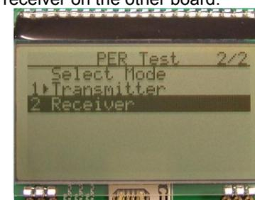
The receiver does not require any further set-up and is now ready to receive packets.
