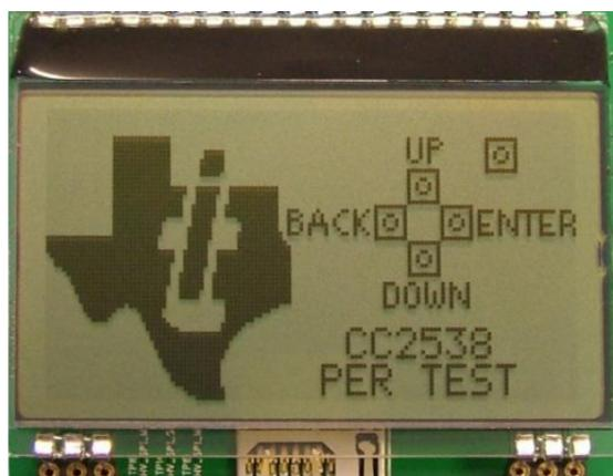
Turn on power with the Main Power switch. You should now see the Texas Instruments logo and a short description of the buttons on the LCD. Pushing any of the five buttons on the board will take you to the main menu.
