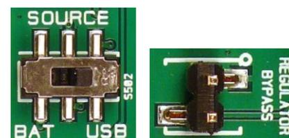
The power source is selected using the Source switch on the left hand side of the SmartRF06EB. In "USB" position, the EM is powered over USB, running at 3.3V. In "BAT" position, the board is powered from batteries or an external source, running at 2.1V. The 2.1V regulator can be bypassed by shorting the pins on the "regulator bypass" jumper. In this case, the EM is powered directly from the external source or batteries.
