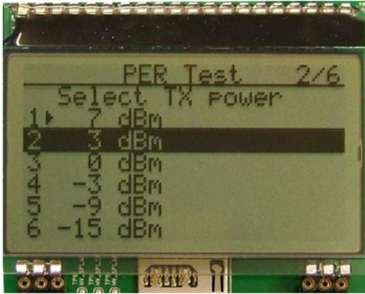
On the transmitter, select desired output power.
