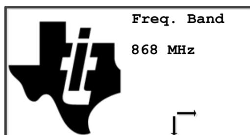
Turn on power with the "POWER" switch to start the pre-programmed Range Test.
