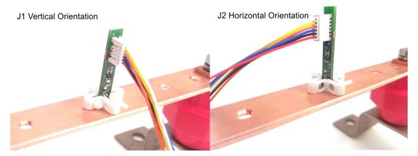
Figure 4. PCB Orientation
