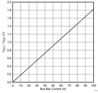
Figure 7. V<sub>OUT</sub> versus Input Current for Vertical Orientation (J1)
