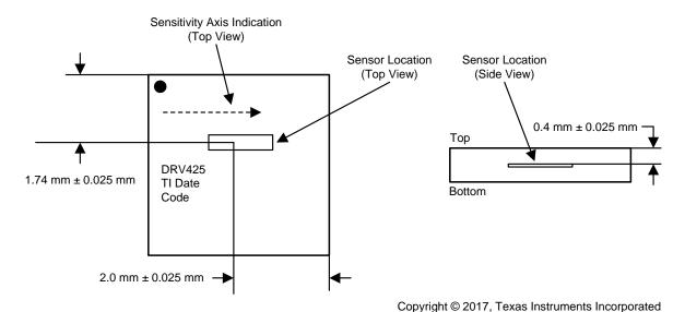
Figure 3. Sensor Location Inside DRV425
