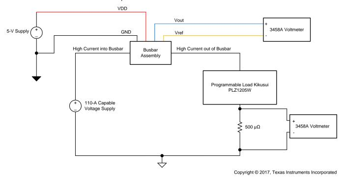
Figure 6. Test Setup Diagram
