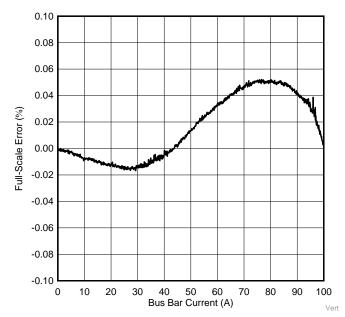
Figure 9. Full-Scale Error versus Current Vertical Orientation (J1)
