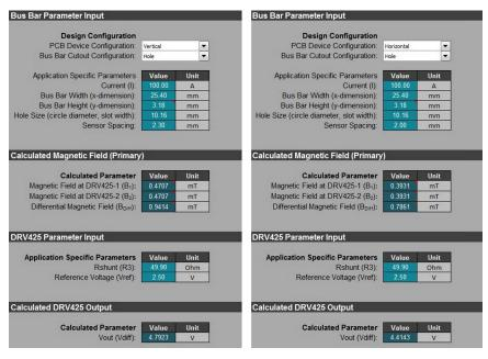
Figure 2. DRV425 Busbar Application Magnetic Field Calculator for Vertical and Horizontal Design
