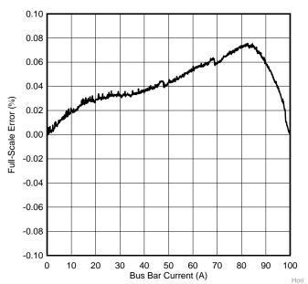
Figure 10. Full-Scale Error versus Current Horizontal Orientation (J2)
