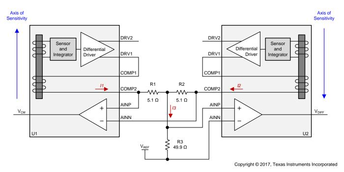
Figure 1. TIPD205 Block Diagram
