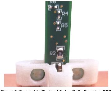
Figure 5. Zoomed-In Photo of Nylon Bolts Securing PCB
