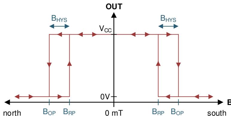
Figure 6-2. Omnipolar Functionality
