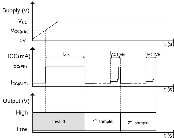
**Figure 6-4. TMAG5328A1D Timing Diagram**
