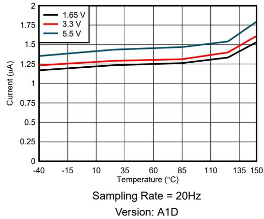
**Figure 5-7. Average I<sub>CC</sub> vs Temperature**
