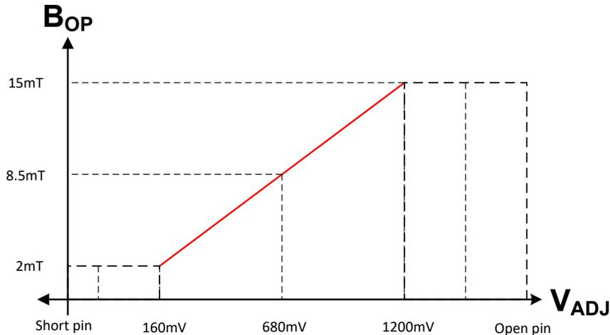
Figure 6-6.  $B_{OP}$  vs  $R_{ADJ}$
