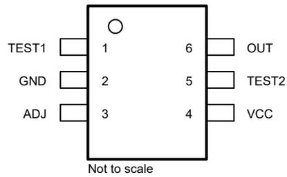
**Figure 4-1. DBV Package 6-Pin SOT-23 Top View**
