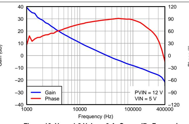
Figure 16. V<sub>OUT</sub>=1.2 V, I<sub>OUT</sub>=3 A, C<sub>OUT1</sub>=47 μF ceramic, C<sub>OUT2</sub>= 330 μF POSCAP, f<sub>SW</sub>=480 kHz
