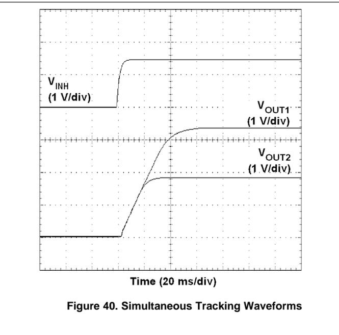
**Figure 40. Simultaneous Tracking Waveforms**
