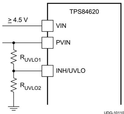
Figure 43. Adjustable PVIN Undervoltage Lockout, (VIN  $\geq 4.5$  V)
