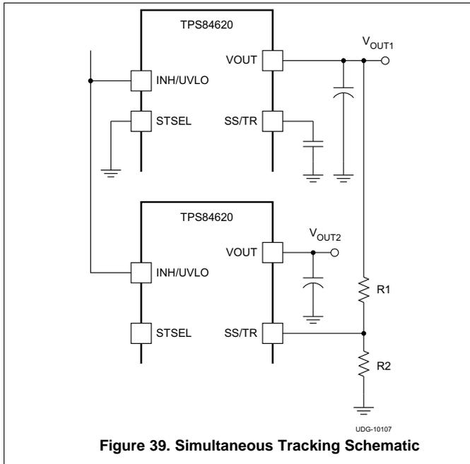
**Figure 39. Simultaneous Tracking Schematic**
