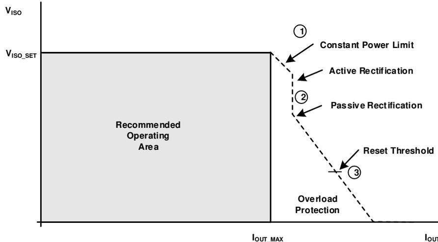
Figure 7-1.  $V_{ISO}$  Load Recommended Operating Area Description
