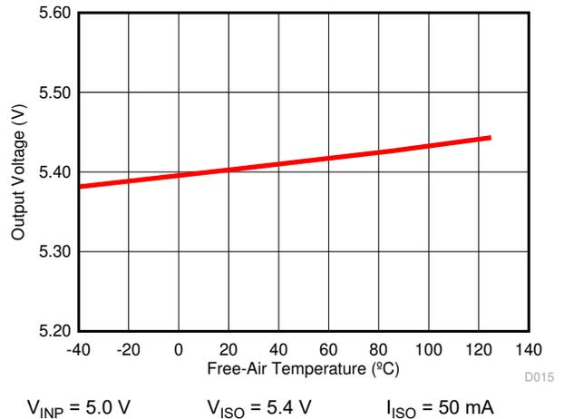
Figure 6-21. Isolated Supply Voltage ( $V_{ISO}$ ) vs Free-Air Temperature
