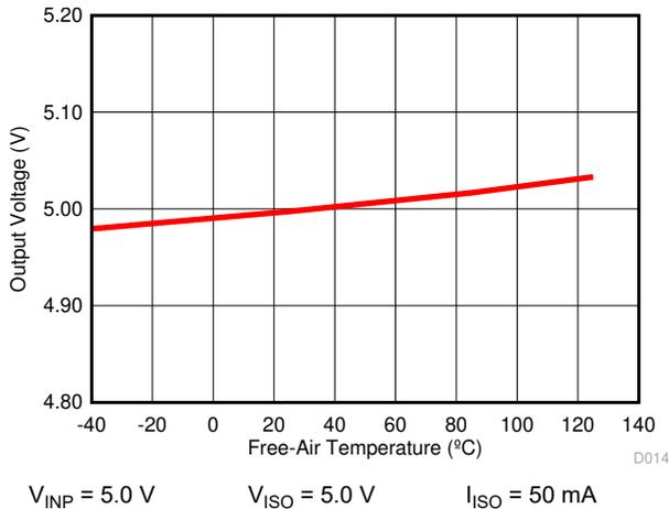
Figure 6-20. Isolated Supply Voltage ( $V_{ISO}$ ) vs Free-Air Temperature
