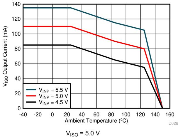
Figure 6-8. Maximum  $V_{ISO}$  Output Current vs. Temperature
