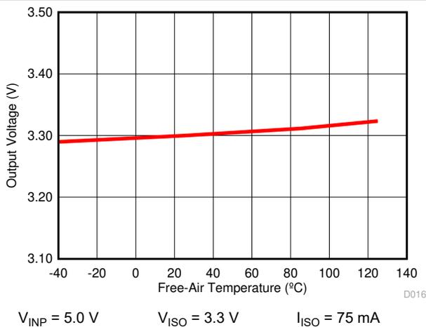
Figure 6-22. Isolated Supply Voltage ( $V_{ISO}$ ) vs Free-Air Temperature
