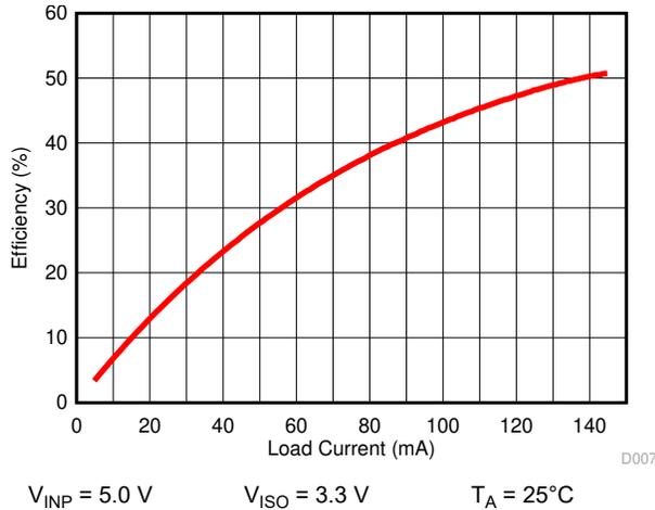
**Figure 6-14. Power Supply Efficiency vs Load Current ( $I_{ISO}$ )**
