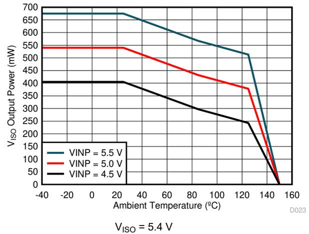
**Figure 6-5. Maximum  $V_{ISO}$  Output Power vs. Temperature**
