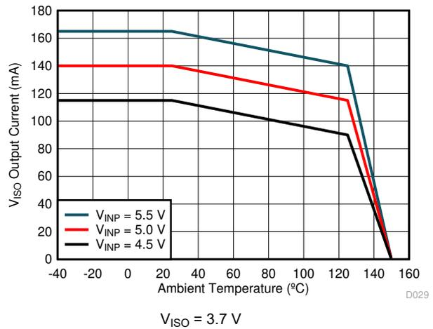
Figure 6-11. Maximum  $V_{ISO}$  Output Current vs. Temperature
