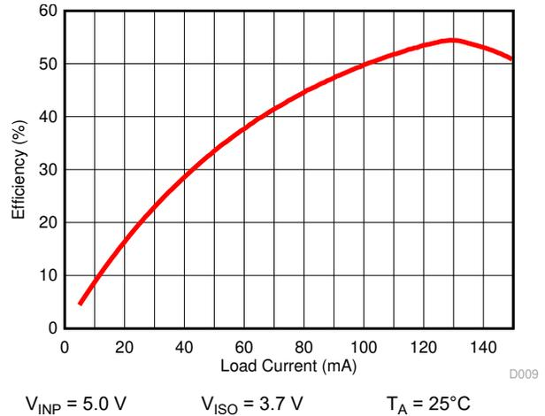
**Figure 6-15. Power Supply Efficiency vs Load Current ( $I_{ISO}$ )**
