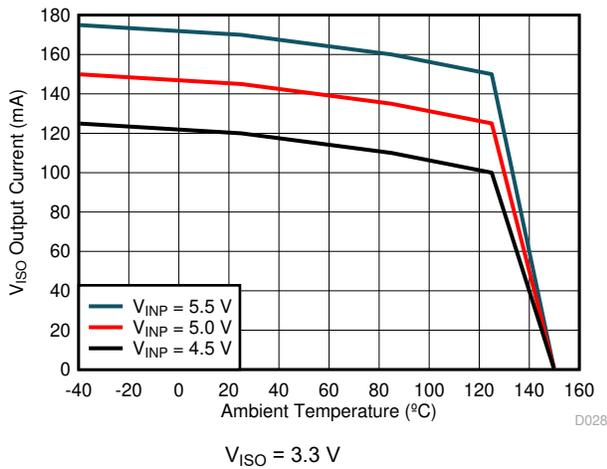
Figure 6-10. Maximum  $V_{ISO}$  Output Current vs. Temperature
