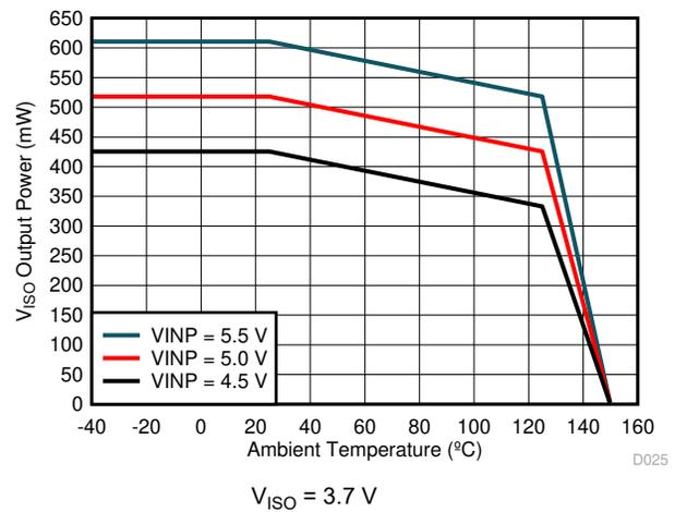
**Figure 6-7. Maximum  $V_{ISO}$  Output Power vs. Temperature**
