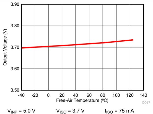
Figure 6-23. Isolated Supply Voltage ( $V_{ISO}$ ) vs Free-Air Temperature
