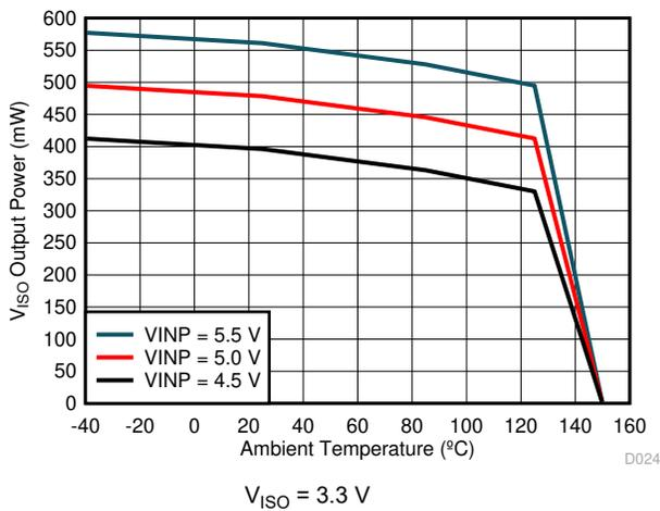
**Figure 6-6. Maximum  $V_{ISO}$  Output Power vs. Temperature**
