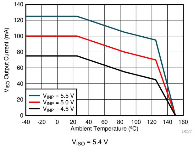
Figure 6-9. Maximum  $V_{ISO}$  Output Current vs. Temperature
