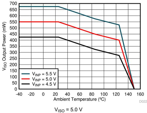
**Figure 6-4. Maximum  $V_{ISO}$  Output Power vs. Temperature**
